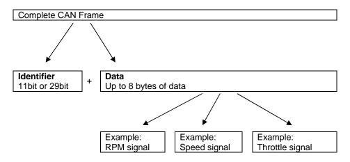
The CAN Display is capable of showing Raw CAN data. Raw CAN data refers to complete CAN frames, showing the identifier and all of the data for each frame in hexadecimal number format.
