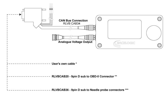
\* The user's own cable must have the D sub wired up as shown on page 4.
