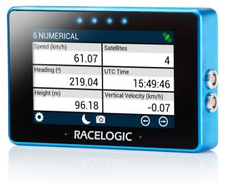
The MFD Touch is ideal for testing where the user needs to monitor one or more parameters live in the vehicle. Up to six GPS derived data parameters can be displayed simultaneously, which are user configurable from the list overleaf, including speed, heading, radius of turn, distance travelled, and numerous brake test channels. The parameters are taken from a standard Racelogic CAN output from the VBOX 3i.
