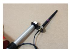
3. Refit telescopic pole to survey bar - routing SMA cable (A8) through to bag interior. Attach female connector on SMA cable (A8) to VBOX Telemetry module (G).
