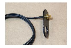
2. Remove telescopic pole from surveying rucksack (A2) and remove the plastic cover from the end of the pole. Secure antenna bracket (A10) telescopic pole using the stainless steel nut provided and screw on the telemetry antenna (A9) to the SMA connector.
