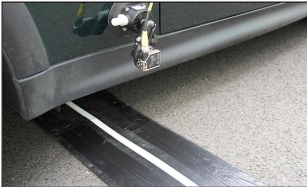
The light barrier is then set facing down towards the ground. This mounting arrangement ensures accurate and consistent strip line detection.
