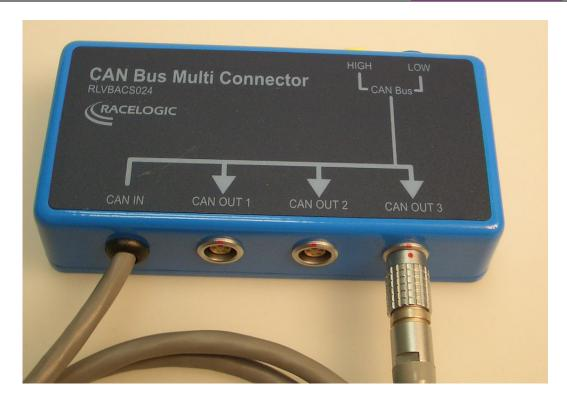
The CAN/5Way Lemo Splitter allows more than one 5 way lemo connection to be connected into one 5 way Lemo socket on a VBOX. This is most commonly used to allow a RS232 and a CAN connection to made into the same socket on a VBOXIII or VBOXII.
