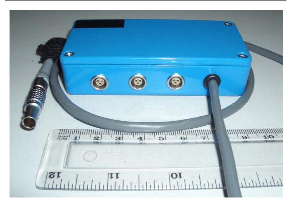
The Digital splitter allows more than one brake trigger to be used at the same time into the Brake trigger input of a VBOX, it also allows an external Start/ Stop logging switch to be connected to the same VBOX socket at the same time.
