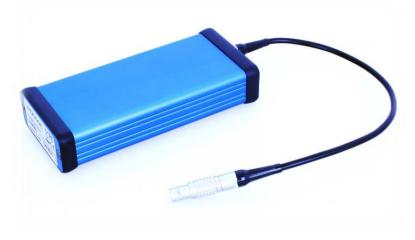
Connected between the vehicle power supply and VBOX 3i, the VBOX Power Backup is capable of storing enough energy to keep the VBOX 3i and connected IMU04 operating during a power supply interruption of up to 20 seconds. The VBOX Power Backup requires an input supply voltage of 10V or higher for over 60 seconds to provide the full 20 seconds of backup power.
