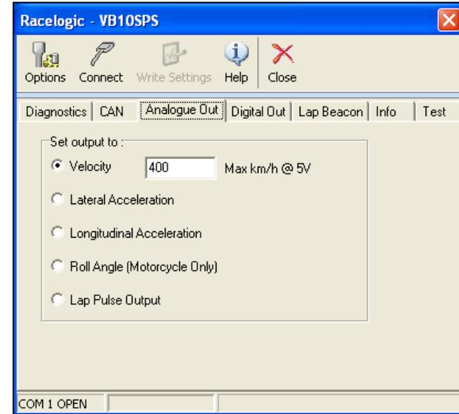
**After making any changes you must click 'Write Settings' for the changes to be programmed into the VB10SPS.**
