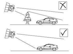
NOTE: VB20SL3 can struggle with maintaining an RTK lock required for Slip, Pitch and Roll measurement if the antennas are placed too close to Roof Bars. If a poor mounting position cannot be avoided then use Ground plane antennas, RLVBACS065.
